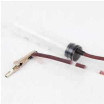
**Step1:** Cut the tube to the length needed. Use the syringe to fill the tube with simulated blood. Use the clamp to close the other end to prevent the blood to spill.
